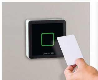
Access control system RFID
