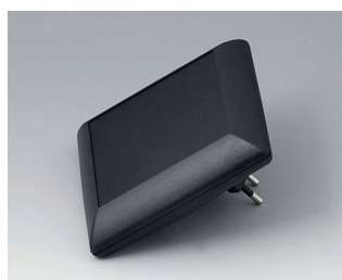
B5013229 ART-CASE S110 F PC+ABS (UL 94 V-0) black RAL 9005 110x110x38mm IP 40
