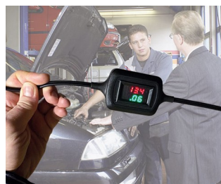
Voltage and current display during trickle charging
