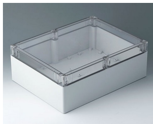
C7030114 IN-BOX ABS/PC (UL 94 HB) light grey RAL 7035 302x232x110mm IP 66, IP 67, IK 07
