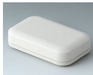
A9421107 EVOTEC 100, Vers. I ASA+PC (UL 94 V-0) off-white RAL 9002 100x62x26mm IP 65 opt., IP 40
