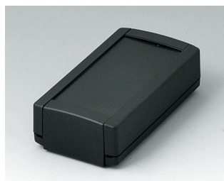
B1040369 TOPTEC 102, Ausf. I ABS (UL 94 HB) schwarz RAL 9005 102x54x30mm IP 40
