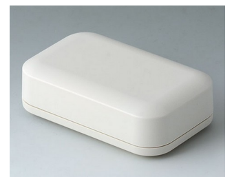
A9423107 EVOTEC 100, Ausf. I ASA+PC (UL 94 V-0) grauweiß RAL 9002 100x62x31mm IP 65 opt., IP 40
