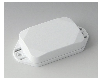
B1822127 MINI-DATA-BOX EF40, flat, with flanges ASA+PC (UL 94 V-0) traffic white RAL 9016 60x40x15mm IP 65 opt., IP 40
