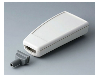
A9066127 SMART-CASE M, Vers. III ABS (UL 94 HB) off-white RAL 9002 96x47x24mm IP 40
