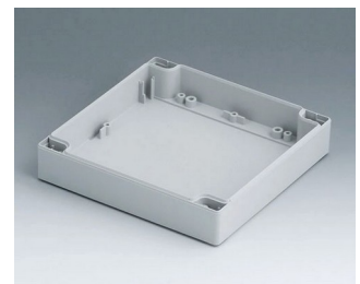
C0161602 Case shell 160, with tongue PC (UL 94 HB) light grey RAL 7035 160x160x30mm
