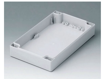
C0122002 Case shell 120, with tongue PC (UL 94 HB) light grey RAL 7035 200x120x30mm
