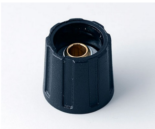
A2516040 ROUND KNOB 16, without line ABS (UL 94 HB) black RAL 9005 16x15mm 4mm
