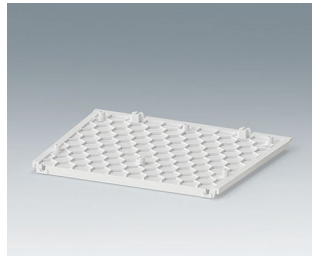
C3602807 Bottom panel ASA+PC (UL 94 V-0) traffic white RAL 9016 188x150x5mm
