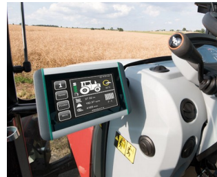
ISOBUS terminal for tractors and self-propelled machines
