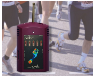
Dynamic pressure measuring between foot and shoe
