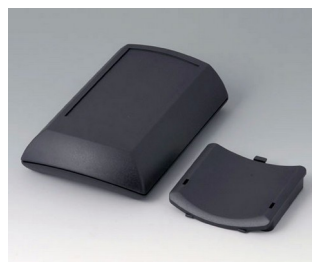
B7010109 ERGO-CASE M, flat ABS (UL 94 HB) black RAL 9005 150x100x40mm IP 54 opt.
