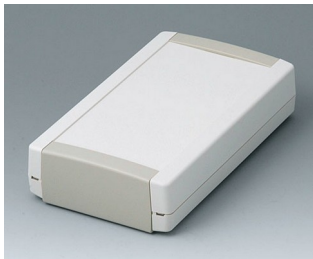
B1075365 TOPTEC 194 F, Vers. I ABS (UL 94 HB) off-white RAL 9002 194x115x46mm IP 40
