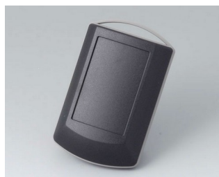
B7040219 ERGO-CASE XS ABS (UL 94 HB) noir RAL 9005 82x56x24mm IP 42
