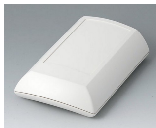
B7010207 ERGO-CASE M, plate ABS (UL 94 HB) gris blanc RAL 9002 150x100x40mm IP 54 opt.
