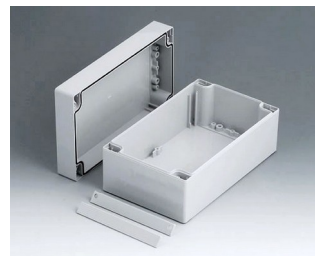
C2112201 ROBUST-BOX 120 LARGE, Vers. I ABS (UL 94 HB) gris clair RAL 7035 200x120x90mm IP 66
