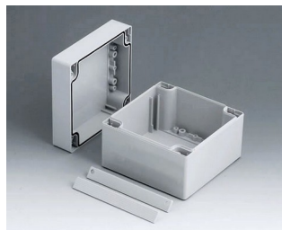
C2112122 ROBUST-BOX 120 LARGE, Vers. II PC (UL 94 HB) gris clair RAL 7035 120x120x90mm IP 66
