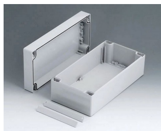
C2112242 ROBUST-BOX 120 LARGE, Vers. II PC (UL 94 HB) gris clair RAL 7035 240x120x90mm IP 66
