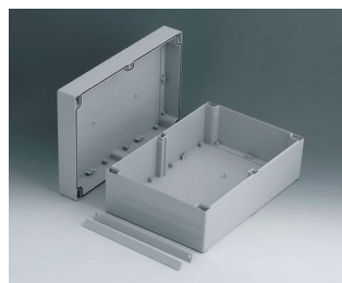
C2420301 ROBUST-BOX 200 LARGE, Vers. I ABS (UL 94 HB) gris clair RAL 7035 300x200x120mm IP 66
