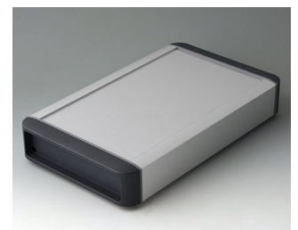
B3407032 SMART-TERMINAL 240 Aluminium AlMgSi 0,5 matt anodised 282x170x50mm IP 54
