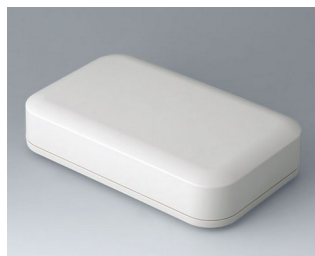
A9461107 EVOTEC 200, Vers. I ASA+PC (UL 94 V-0) off-white RAL 9002 200x124x45mm IP 65 opt., IP 40
