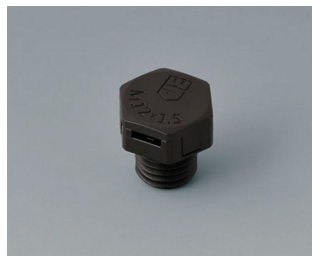
C2304969 Pressure equalisation element M12x1.5 PA 6 (UL 94 V-0) black RAL 9005
