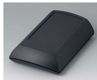
B7010209 ERGO-CASE M, flat ABS (UL 94 HB) black RAL 9005 150x100x40mm IP 54 opt.
