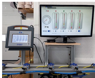
Monitoring system for cleaning nozzles
