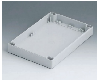
C0162402 Case shell 160, with tongue PC (UL 94 HB) light grey RAL 7035 240x160x30mm
