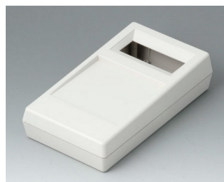
A9061117 HAND-HELD-BOX N, Vers. II ABS (UL 94 HB) off-white RAL 9002 180x100x44mm
