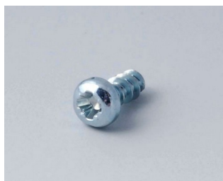
A0305031 Self-tapping screws 2.5 x 6 mm (PZ1)
