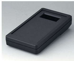
A9073409 DATEC-MOBIL-BOX S, Vers. IV ABS (UL 94 HB) black RAL 9005 152x83x33,5mm IP 65 opt.
