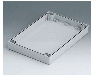
C1162401 Case shell 160, with groove ABS (UL 94 HB) light grey RAL 7035 240x160x30mm
