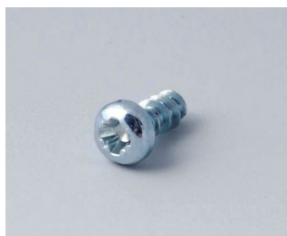
A0305031 Self-tapping screws 2.5 x 6 mm (PZ1)
