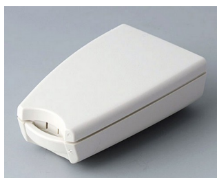
A9064107 SMART-CASE XS АБС (UL 94 HB) белый RAL 9002 58x35,6x19mm IP 40
