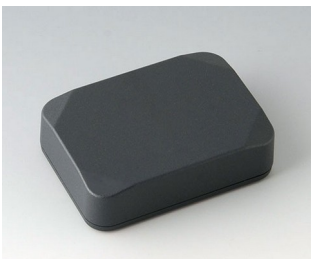
B1824218 MINI-DATA-BOX E50, high ASA+PC (UL 94 V-0) anthracite grey RAL 7016 70x50x20mm IP 65 opt., IP 40
