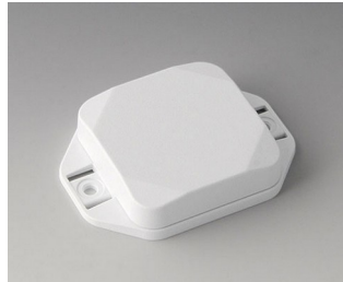
B1804127 MINI-DATA-BOX SF50, flat, with flanges ASA+PC (UL 94 V-0) traffic white RAL 9016 50x50x15mm IP 65 opt., IP 40
