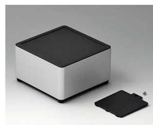
ES126059 SYNERGY S120 Aluminium AlMgSi 0.5 matt anodised 120x120x70mm IP 40
