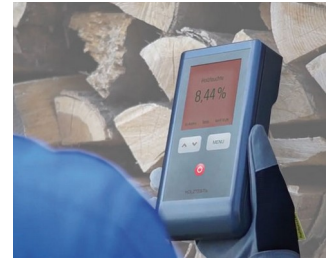
Wood moisture measuring device
