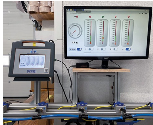
Monitoring system for cleaning nozzles
