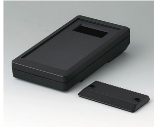
A9073309 DATEC-MOBIL-BOX S, Vers. III ABS (UL 94 HB) black RAL 9005 152x83x33.5mm IP 65 opt.
