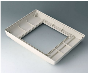
B4046767 Bottom part L high, version II ABS (UL 94 HB) off-white RAL 9002 275x195x36.5mm IP 54 opt.
