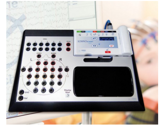
Stationary system for long-term EEG recordings
