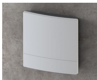
B3222201 NET-BOX 220, Vers. II ASA+PC (UL 94 V-0) light grey RAL 7035 220x220x50.5mm IP 65 opt.
