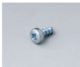
A0306031 Self-tapping screws 3 x 6 mm (PZ1)
