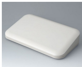
A9485107 EVOTEC 250, Vers. II ASA+PC (UL 94 V-0) off-white RAL 9002 250x155x54mm IP 65 opt., IP 40
