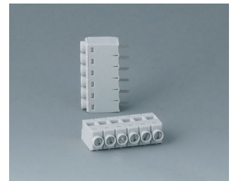
B6607111 Terminal block, block 5.0 PA 68 (UL 94 V-0)
